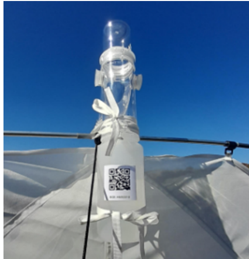
Figure 7. Example of a collection tube correctly placed and secured in the trap using the white straps around it.
