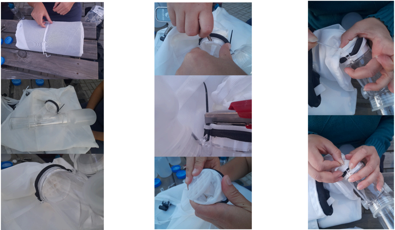
Figure 4. Example of how to remove the plastic grid included in the Malaise trap.
