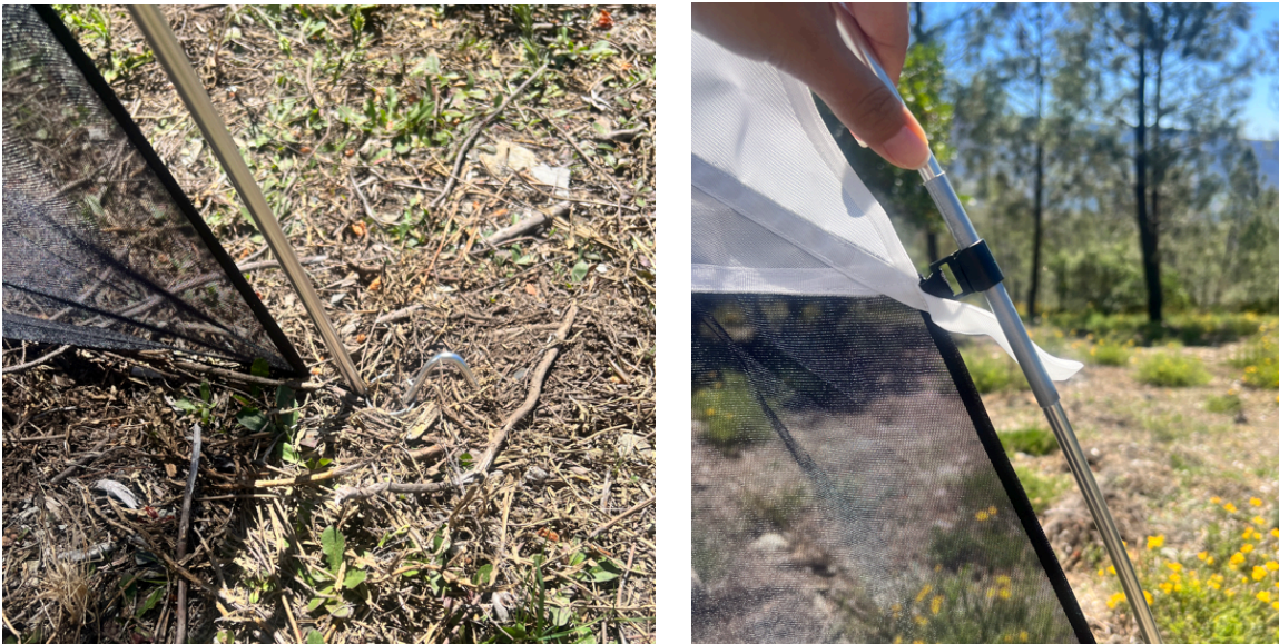
Figure 5. Metal stack/peg placed at one of the extremes of the Malaise trap (left). Gray tape placed in the joints of the trap metal structure for reinforcement (right).
