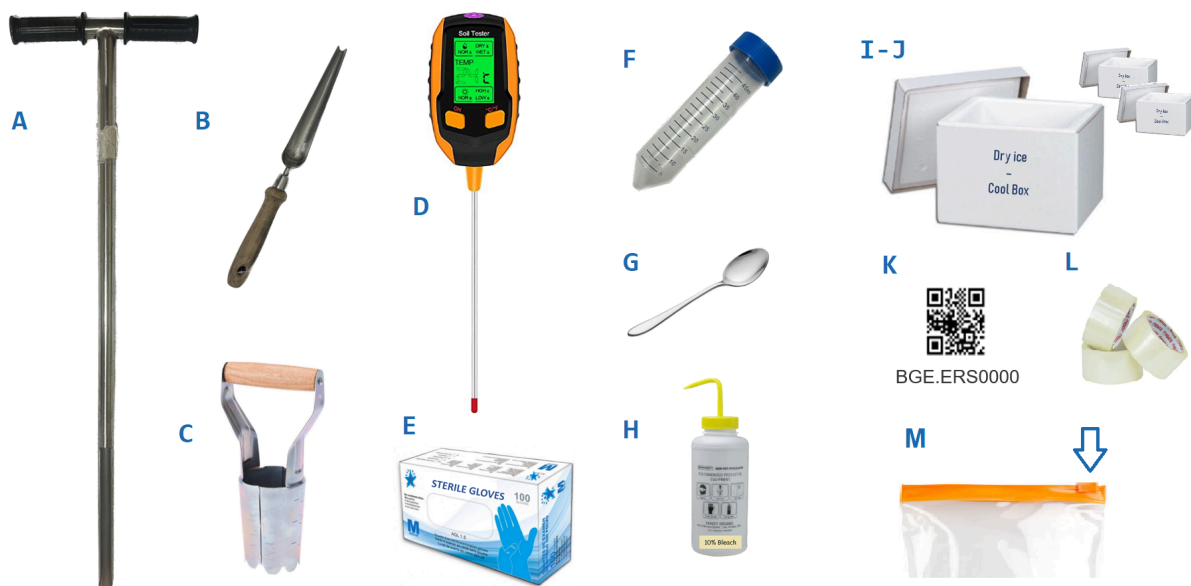
Figure 3. Materials needed for soil sampling. Letters refer to the materials list.
