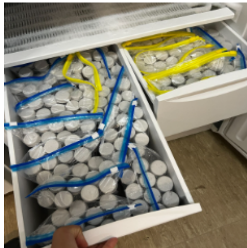
Figure 4. Space occupation of 240 tubes in -20°C freezer drawers. Total core's samples of each replicate are contained in separated zip hermetic bags (10 tubes per bag).
